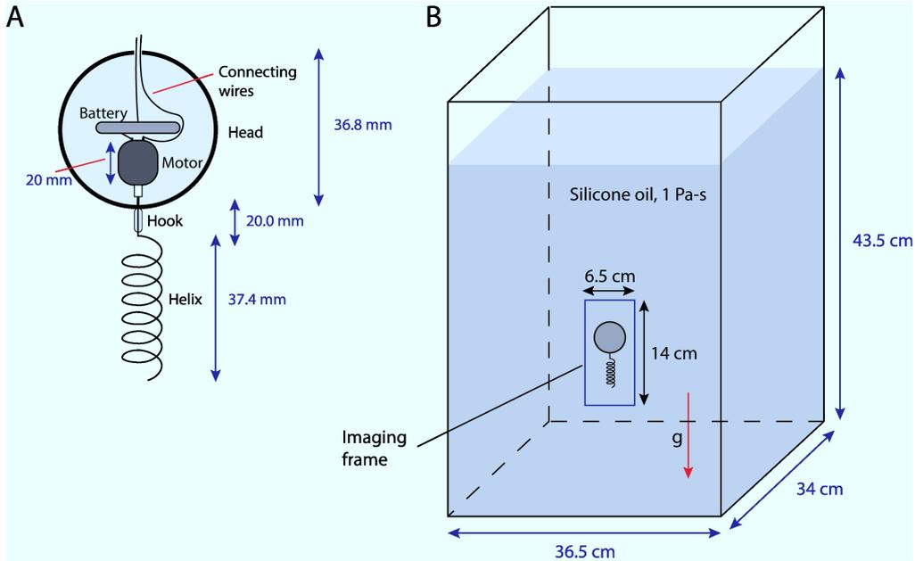
FIGURE 1. (A) A schematic of the model bacterium used in the experiments. (B) Dimensions of the tank and the approximate location of the bot during a run.
