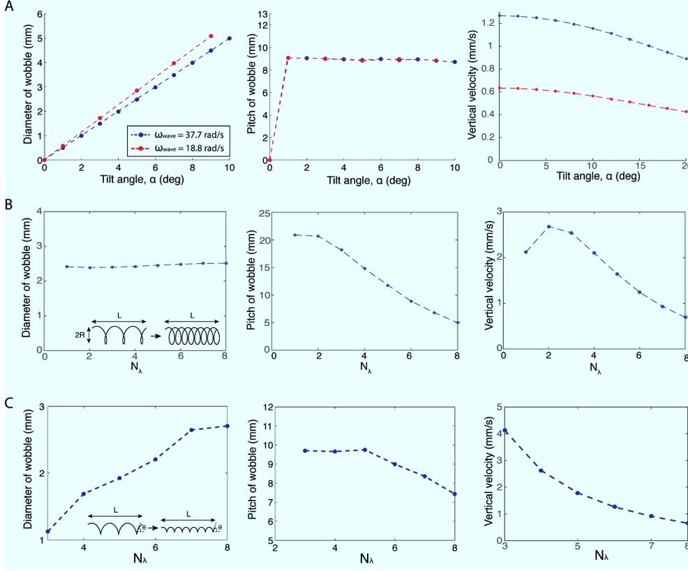
FIGURE 4. The figure plots the radius, pitch and the vertical velocity component for (A) varying tilt angles ( $\alpha$ ) (B) varying number of helical turns with  $L$  and  $R$  fixed, and (C) varying number of helical turns with  $L_c$  and  $\theta$  fixed, and therefore  $L$  is also fixed.
